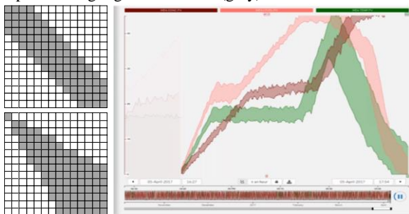
Figure 5: DTW can be constrained by only allowing it to visit the cells marked in gray. In left.top we show a classic fixed warping constraint window, and in left.bottom we show a growing warping constraint window, that is designed to model accumulating “drift” over time. The need for this growing constraint is reflected in this commercial dataset ( right ).
